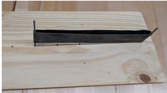
Figure 4. An image of the testing apparatus that produces variable levels of inward radial force.
