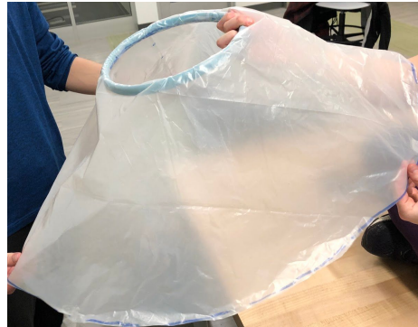
Figure 3. An image of the conical shape film design. The top of the image is where the interior ring would be located and the bottom of the image is where the expanding exterior ring would be located
