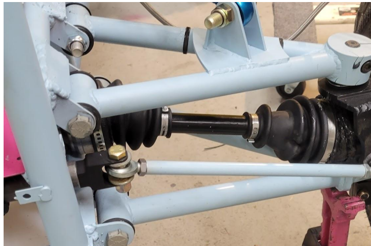
Figure 21: The outer CV joints boot disconnected from the joint causing grease to escape and dirt and mud to get it.
