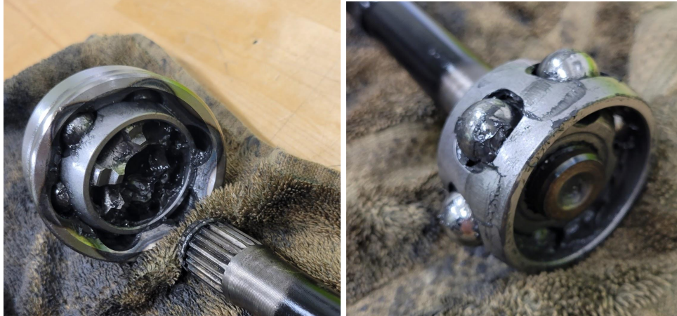
Figure 16: These images represent the two joints from the Sixity axle. The image on the left shows the internal components of the Rzeppa joint, while the image on the right shows the internal components of the plunging joint, which is a double offset joint.
