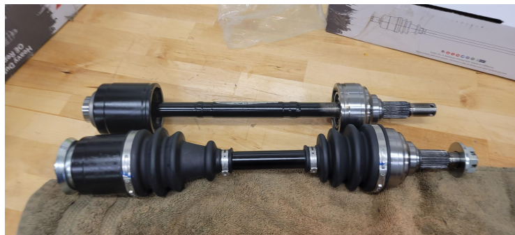
Figure 15: The axle on the top is the Sixity axle that was ordered to verify it would work in the Baja vehicle. It was deconstructed and taken apart to get a better understanding of its working components. Once it was deemed it could work, five more were ordered for the car (one extra is case of issues), one of which is the axle on the bottom.
