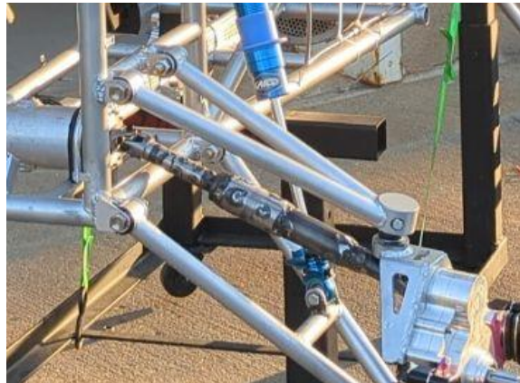
Figure 14: Half shafts for the 2021-2022 Racing Vehicle. Consists of two universal joints with a splined slip joint in the middle. Served as the inspiration for one of the designs for the 2022-2023 Racing Vehicle.
