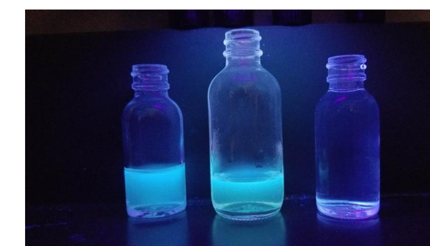
Figure 7: GQD solutions using an industrial kiln as the heating source with the left solution being 2g Glutamine to 10 mL of water and the middle solution being 4g Glutamine to 10mL water. Water is shown on the right for reference
