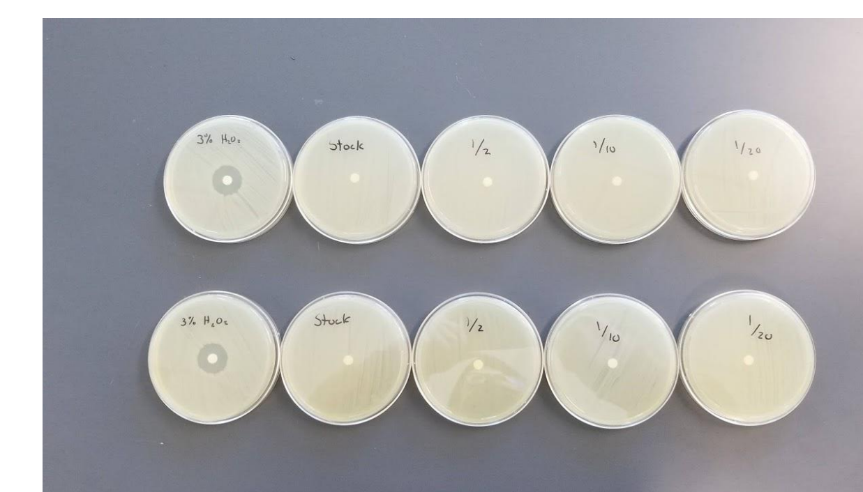
Figure 9 (Right): Antibacterial testing using E.coli grown on agar covered petri dishes. Hydrogen Peroxide is used as a control on the left with GQD solutions ranging from stock concentration to 1/20 th the concentration. No ring of inhibition is seen from the GQD samples.
