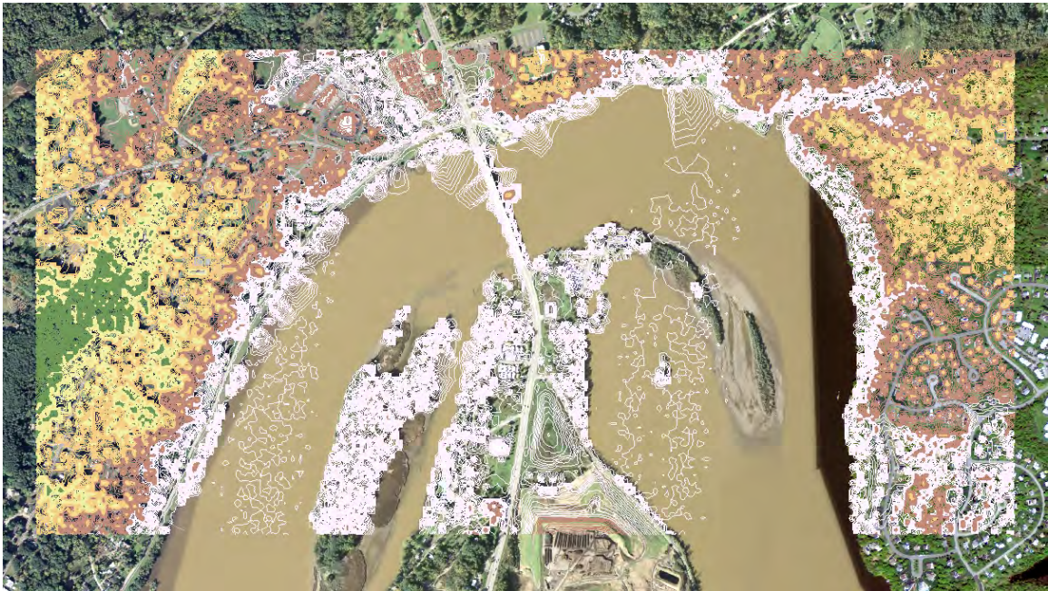
LiDAR image analysis of a curved segment along the Mohawk river superimposed over a GEO TIFF image of the same location.
